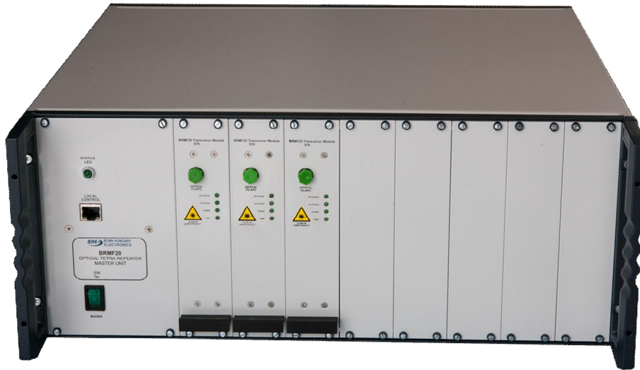
Picture of base station side BRMF20 Master repeater with 6 (max 8) optical outputs
